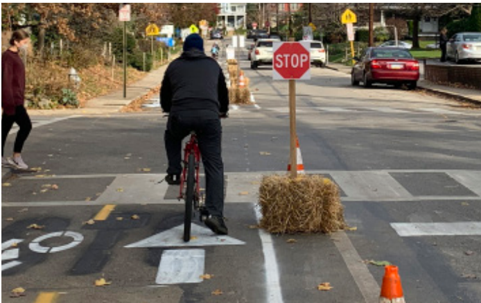
The Wheels on Windsor project in Narberth Borough, PA included a two-block bike lane protected using hay bales and traffic cones.
